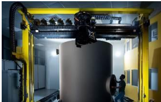
PIC. 10: LARGIX’S ROBOTIC PRODUCTION PLATFORM CAN PRODUCE 3D-PRINTED INDUSTRIAL ITEMS FOR INDUSTRY INCLUDING ROOM-SIZED STORAGE TANKS FOR CHEMICALS (LARGIX)
