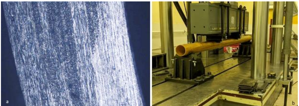
Fig. 1. – a - Microstructure and b - appearance of glass-basalt-plastic composite pipes during strength tests
